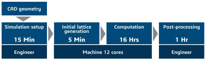
Based on High-fidelity Transient CFD Simulation conducted for the AIAA 1st High Lift Prediction Workshop
